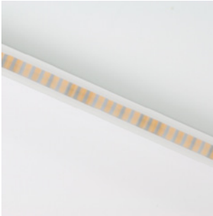
S 14° lens (KCLN-01D) 14° beam linear lens, co-extruded PMMA W12.8/H20mm (W0.50"/H0.79")
